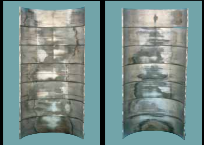
Comparison photos of lower main bearings show that after 370,000 km of severe service under high loads, the wear control of Mobil Delvac 1 ESP 0W-40 (on right) was equal to or better than a leading 15W-40 lubricant (on left).
