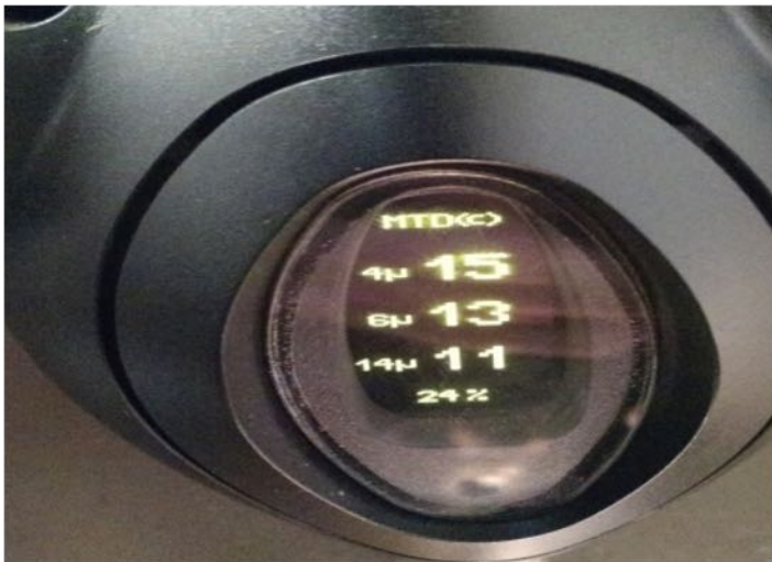
An inline laser particle counter provided real-time oil analysis
