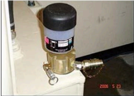
Figure 1. BSF kit installed on a hydraulic oil reservoir
