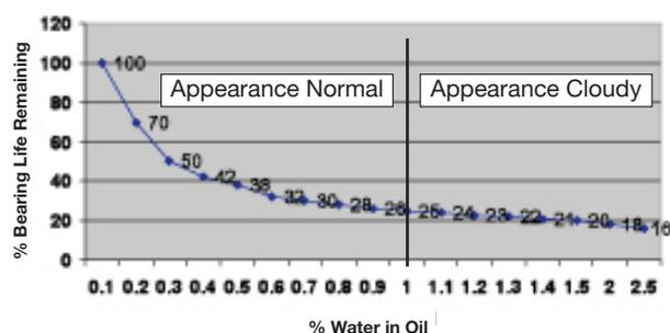
Maintaining minimum water levels is a must. The most common methods of continuous water removal are centrifugal purification for large amounts of water and vacuum dehydration (polishing) for concentrations under 400 ppm.
